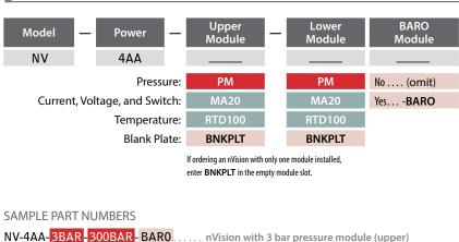
nVision with 3 bar pressure module (upper) and 300 bar pressure module (lower); and a BARO module option.
