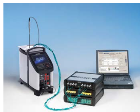
ASM A models connected to the ASM B model, in order to obtain 24 channels. The JOFRA RTC calibrator is used as a dry-block with the reference sensor connected to the reference input of the ATC, all controlled by JOFRA CAL.
